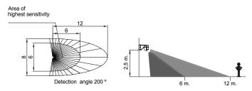
It must be taken into account when installing the MULTIMAT that detection takes place when the detection beams are crossed; therefore, if the heat source to be detected is moving parallel to the beams, detection will be produced at a smaller distance since it will not cross the beams until it is very close to the apparatus.
